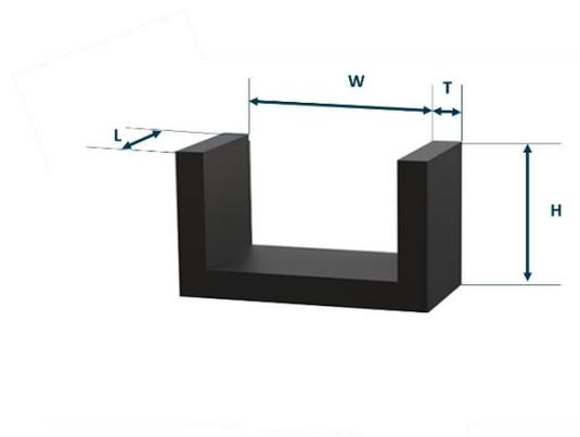
Figure 13: definition of dimensions of shields.
