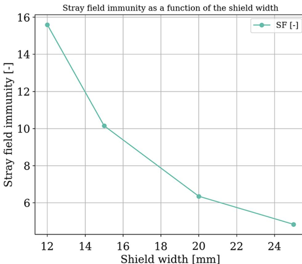
Figure 18: Shielding factor versus shield width.
