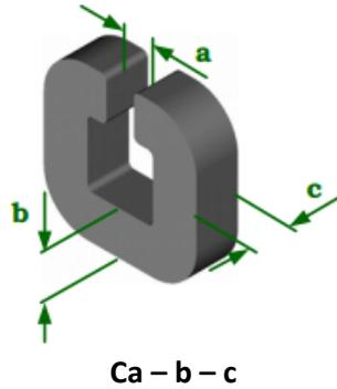
Figure 41: Ordering convention for laminated cores.
