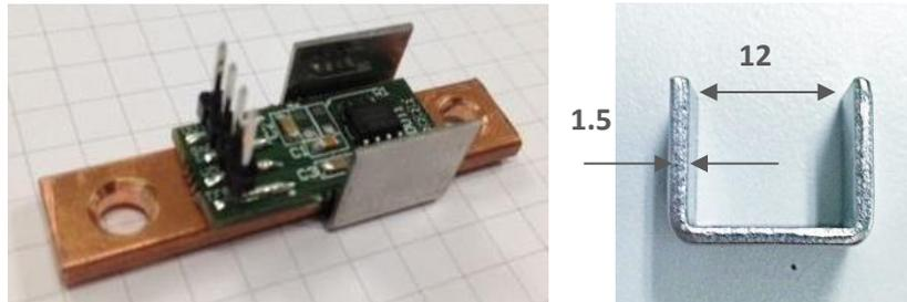
Figure 31: Demonstrator based on MLX91208 VHF sensor and U12 shield with 1.5mm thickness.
