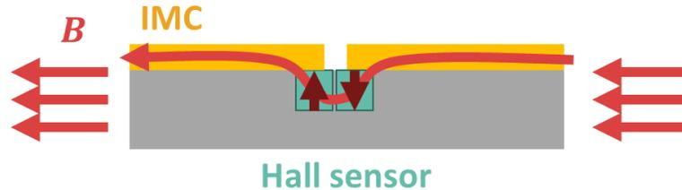
Figure 8: IMC and field bending. Any field in the Z direction is rejected by the differential sensing.
