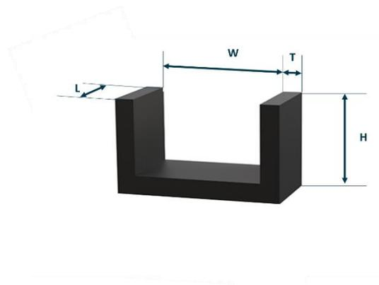
Figure 13: definition of dimensions of shields.
