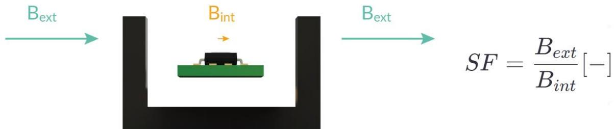
Figure 17: Shield factor definition
