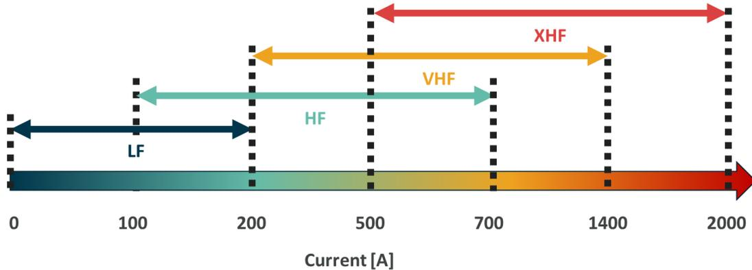
Figure 11: Optimal IMC configuration for different current ranges. Saturation of shields should also be considered. Melexis offers an online simulator tool, to choose the most optimized solution for a current sensing application, the [current sensor simulator](#).
