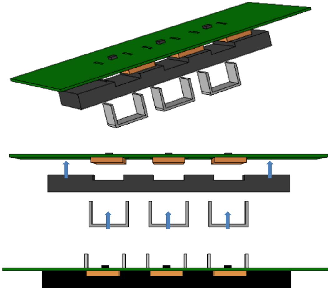
Figure 39: Assembly with pre-molded plastic case.
