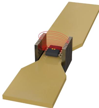
Figure 15: Necked-down bus bar example.
