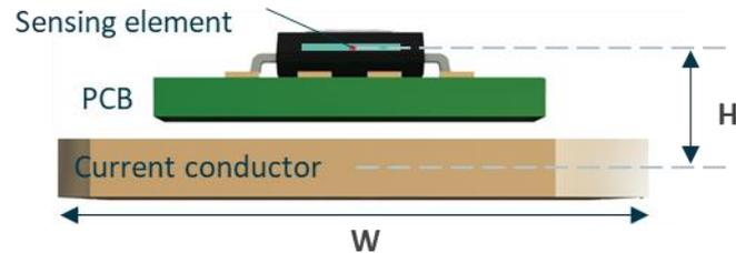
Figure 14: dimensions on sensor without shield.
