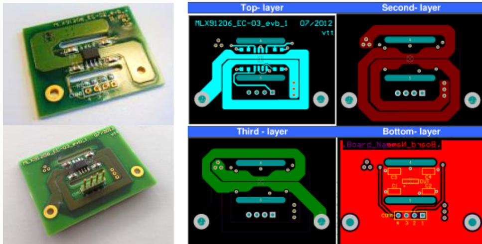
Figure 25: PCB layout example for very high sensitivity with 6 windings on 3 layers.
