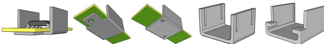
Figure 38: Several solutions for shield assembly.
