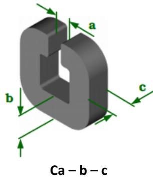
Figure 41: Ordering convention for laminated cores.
