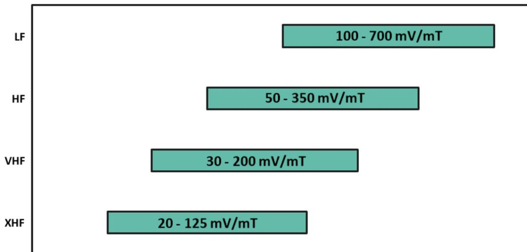
Figure 9: Sensitivity range of each IMC version.
