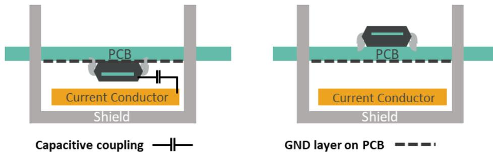
Figure 23: Current sensing structure. Expanded Ground Layer on PCB in order to reduce the parasitic coupling capacitance (coming from voltage transients).
