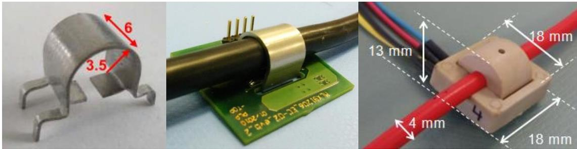
Figure 35: Implementation examples (monolithic and two-part shield in plastic housing).
