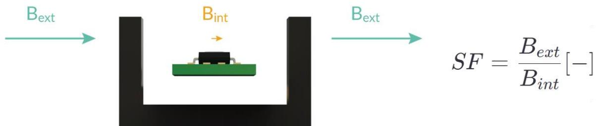
Figure 17: Shield factor definition
