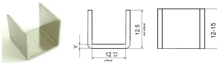
Figure 29: Shield dimensions.
