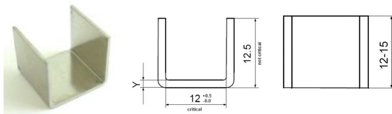
Figure 29: Shield dimensions.
