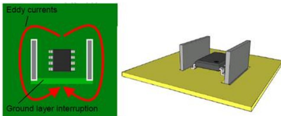
Figure 24: Current Sensing Structure – Designing the Ground Layer on the PCB such that Eddy Currents circulations is interrupted
