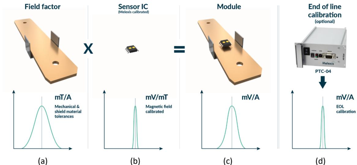
Figure 42: Sum of error of sensor and mechanical assembly. We can see that the mechanical assembly (a) introduces an error that will affect the total error (c). An end of line calibration (d) will lower again the error to the value of the sensor after fabrication (b).
