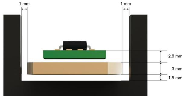
Figure 12: Shield and sensor assembly, with standard spacings.
