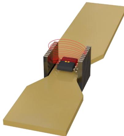
Figure 15: Necked-down bus bar example.
