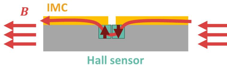
Figure 8: IMC and field bending. Any field in the Z direction is rejected by the differential sensing.
