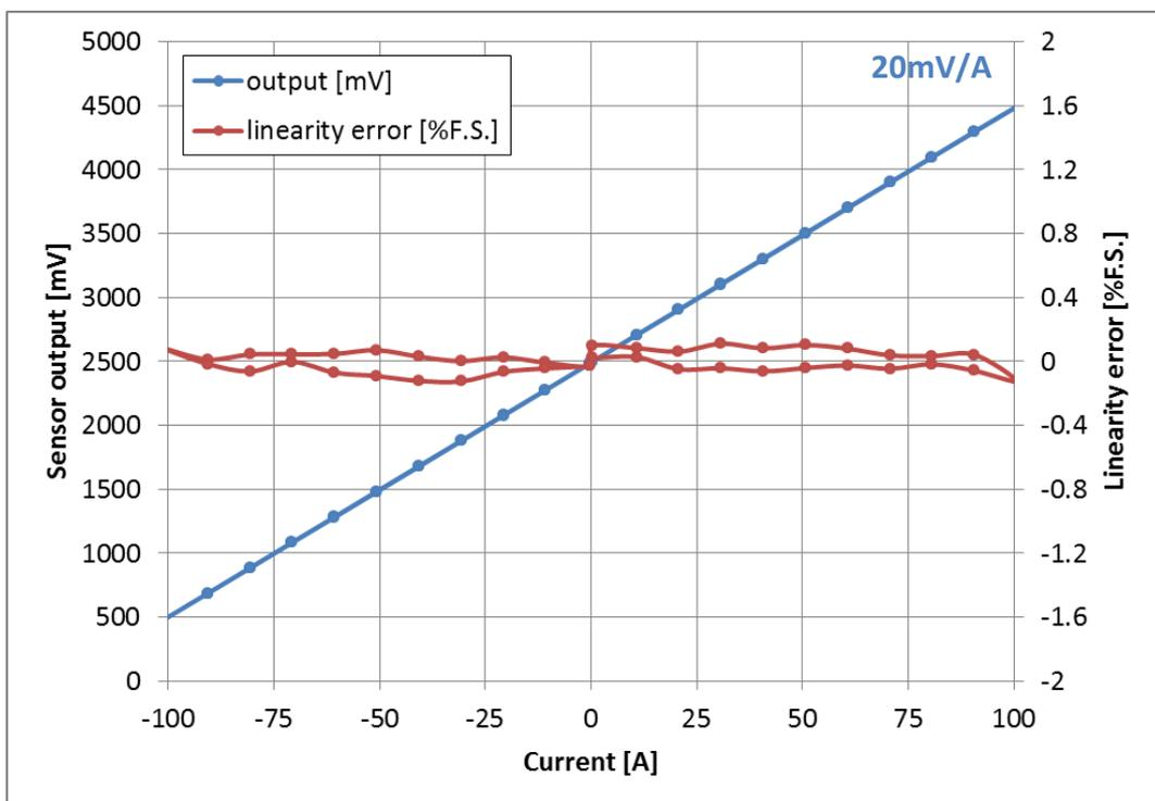
Figure 30: Typical output and non-linearity of a sensor calibrated for  $\pm 100A$ .
