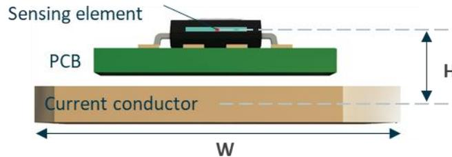
Figure 14: dimensions on sensor without shield.
