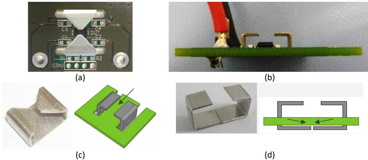
Figure 26: Top (a) and side (b) view of the full system. (c) Shield in one piece inserted through slots on the PCB edge. and (d) shield in two parts inserted in PCB slits and assembled together.
