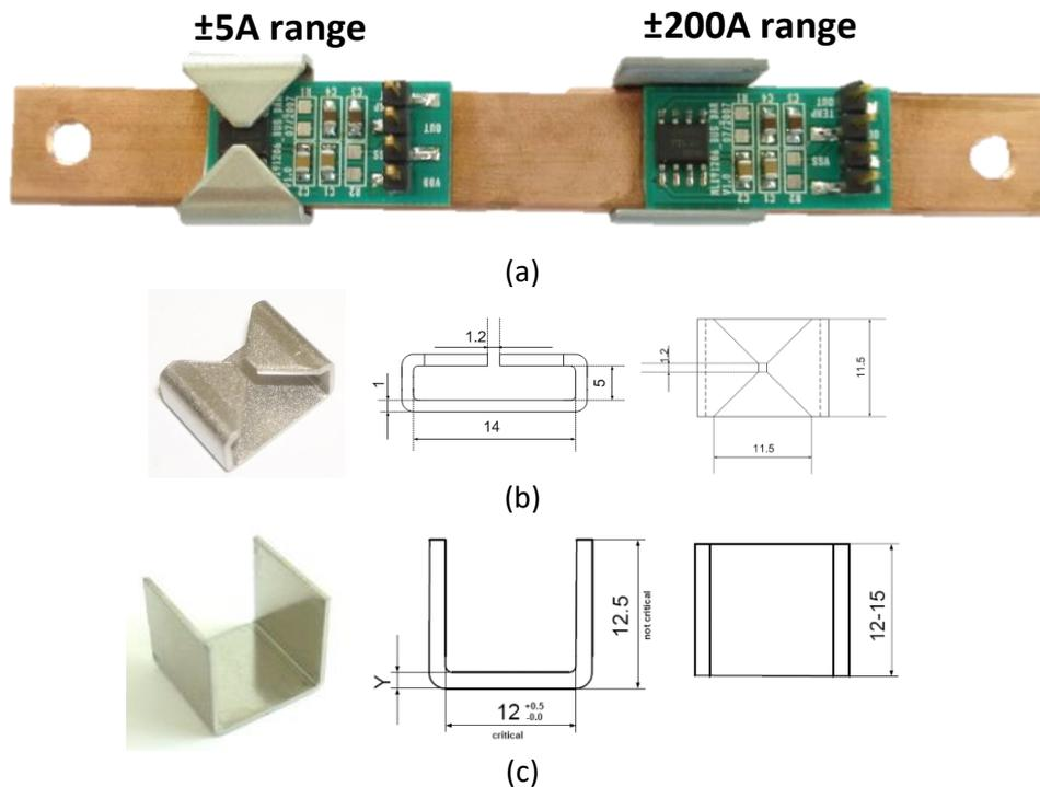
Figure 33: (a) Assembly. Images and sections for (b) closed shield and (c) U-shaped shield.
