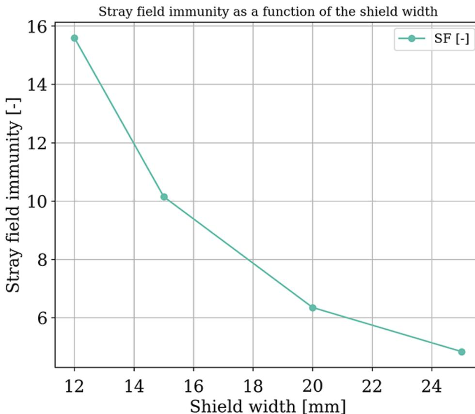
Figure 18: Shielding factor versus shield width.
