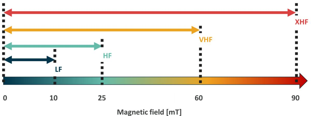
Figure 10: Linearity range for different IMC configurations.
