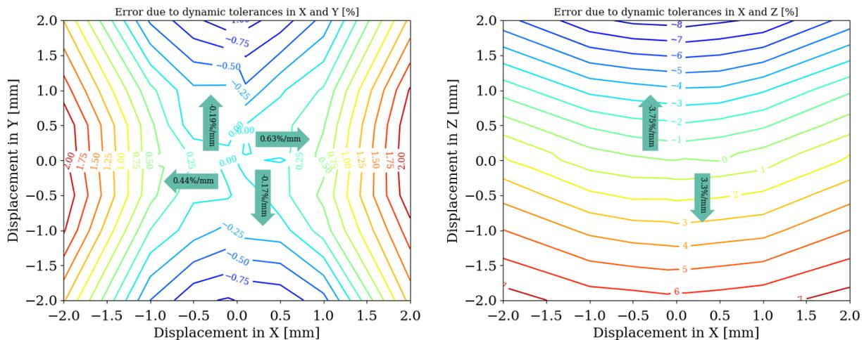
Figure 19: Effect of mechanical vibrations on the sensitivity.
