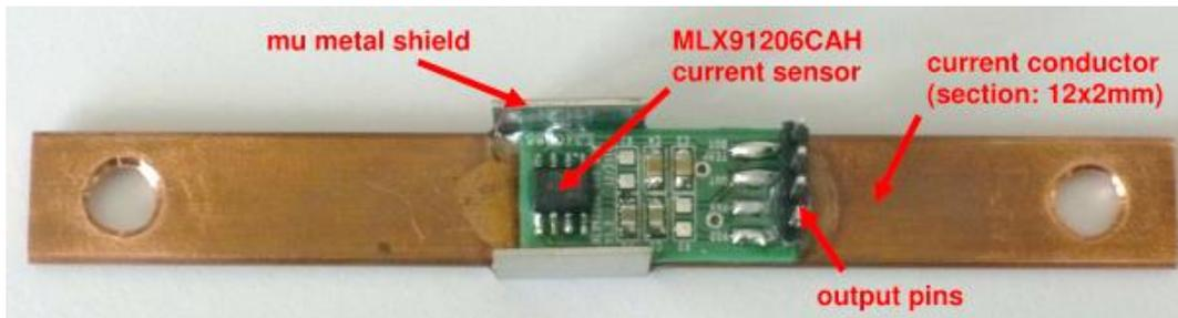
Figure 28: Demonstrator based on MLX91206 HF sensor and U12 shield with 0.8mm thickness.
