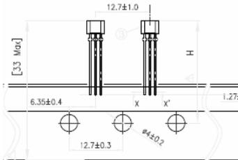
Pitch 1.27mm - Max lead length after cut = 11.5mm
