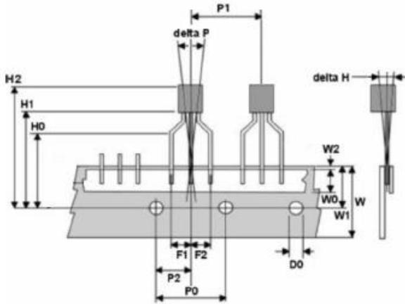
**Meax Lead Length after cut = 10mm.**
