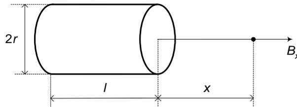
*Note 1: Knowing that the magnet used for this measurement is covered with nickel coating (reducing the  $B_r$ ), and taking into account the magnet's tolerances and external magnetic disturbances, practical measurements show results quite close to the theoretical formula.*
