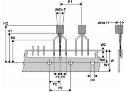
Pitch 2.54mm - Maxx Lead Length after cut = 10mm.
