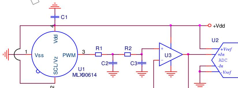
With  $R1=47k$ ,  $R2=470k$ ,  $C2=C3=1\mu F$ , the ripple (again at 5V, 50%, 1kHz) seen by the ADC will be less than 20  $\mu V$ . Note that this ripple reduction comes with significantly increased settling time (3 seconds for this case). Certainly, a cost-effective approach might be to use a first order RC network between the MLX90614 and the ADC in conjunction with digital filtering of the ADC output.
