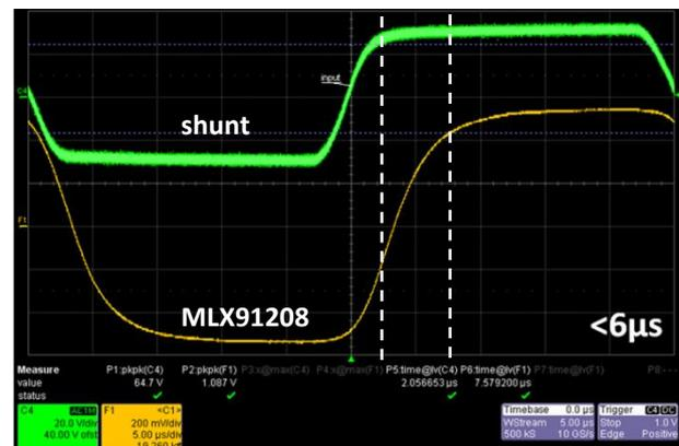
Figure 9: Response time with noise filter ON.
