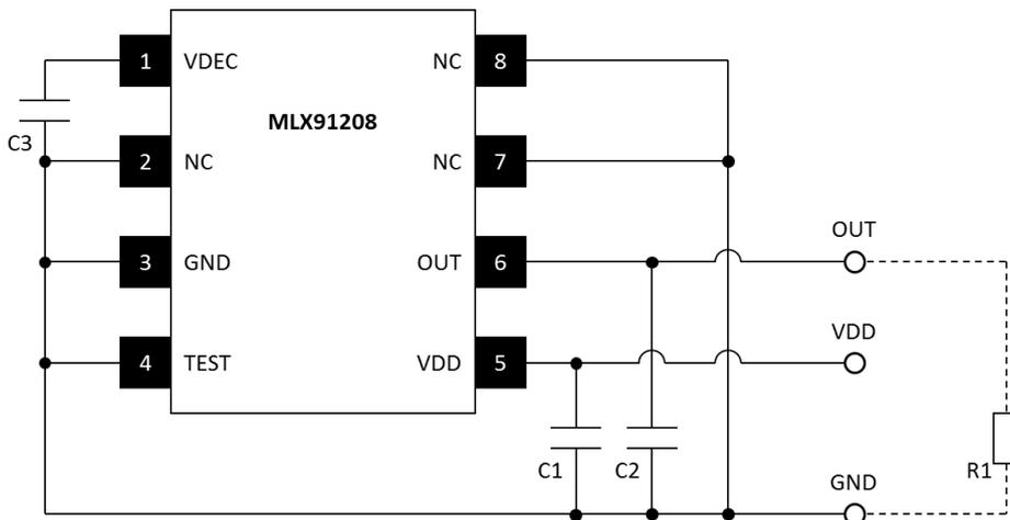
Figure 4: Diagnostic low/ Pull-down resistors
