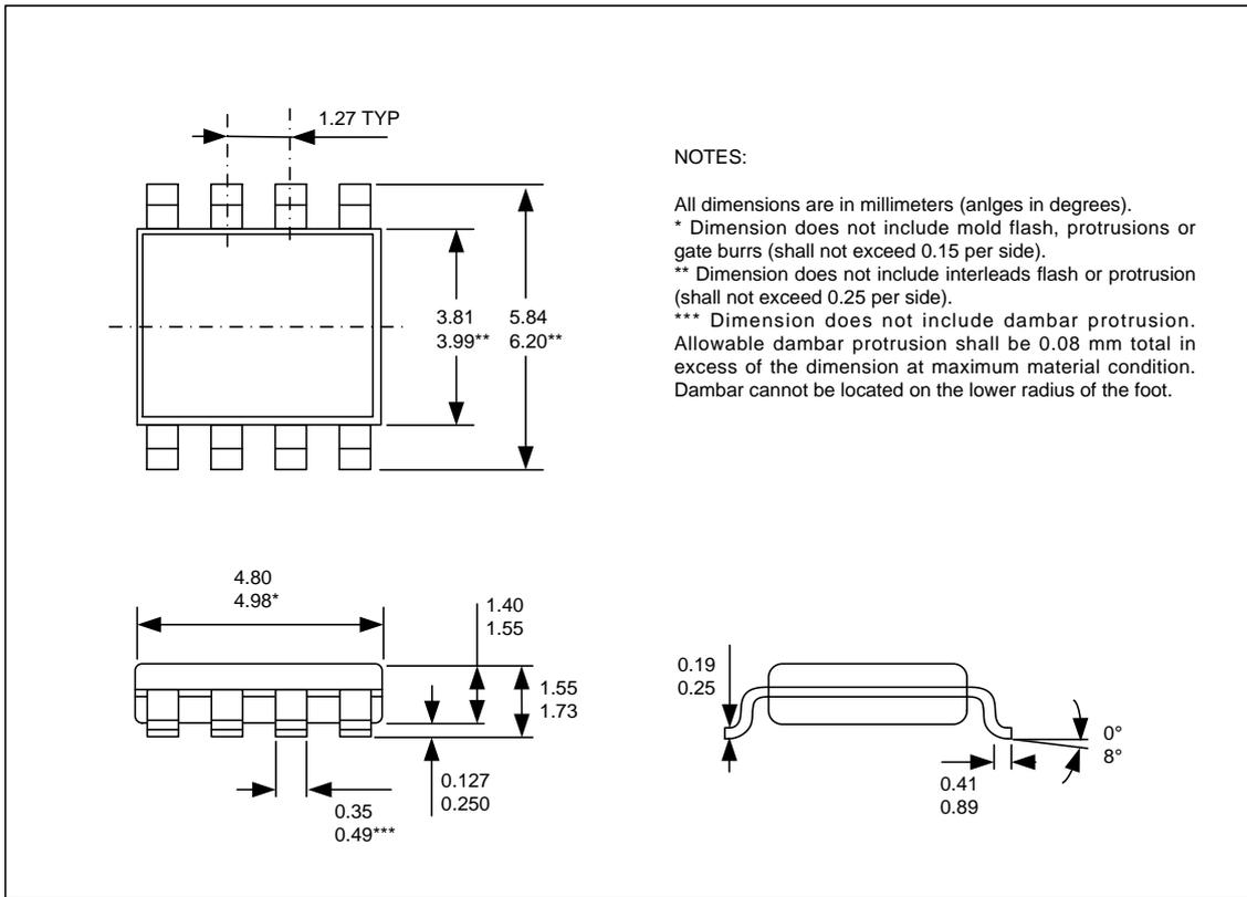
Figure 10: SOIC-8 Package dimensions
