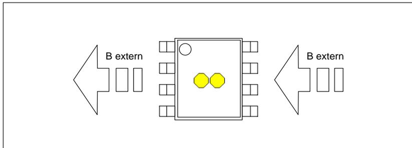
Figure 14: IMC position and geometry high-field version
