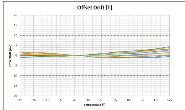
Figure 6: Thermal offset drift.
