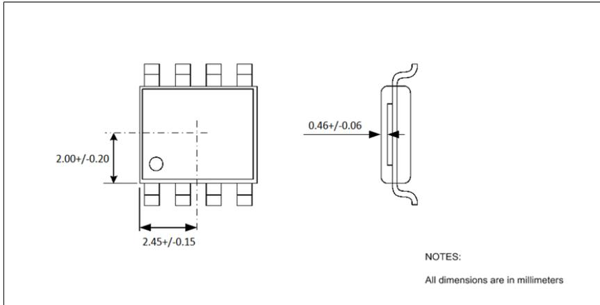
Figure 12: SOIC-8 Hall Plate positioning
