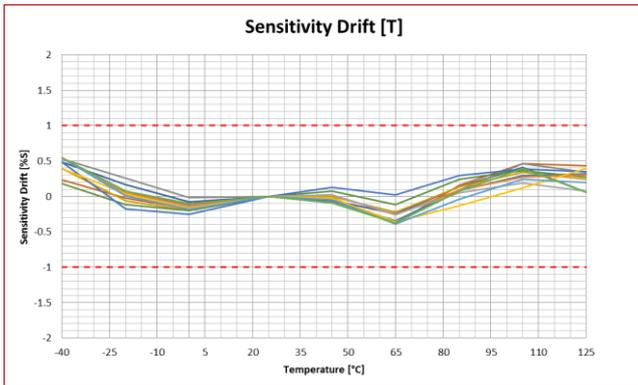
Figure 5: Thermal sensitivity drift.
