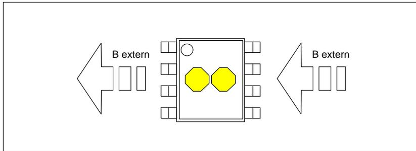
Figure 13: IMC position and geometry for low-field version
