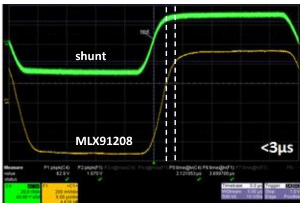
Figure 8: Response time with noise filter OFF.
