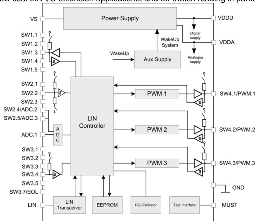
Figure 3 - Block diagram MLX80104
