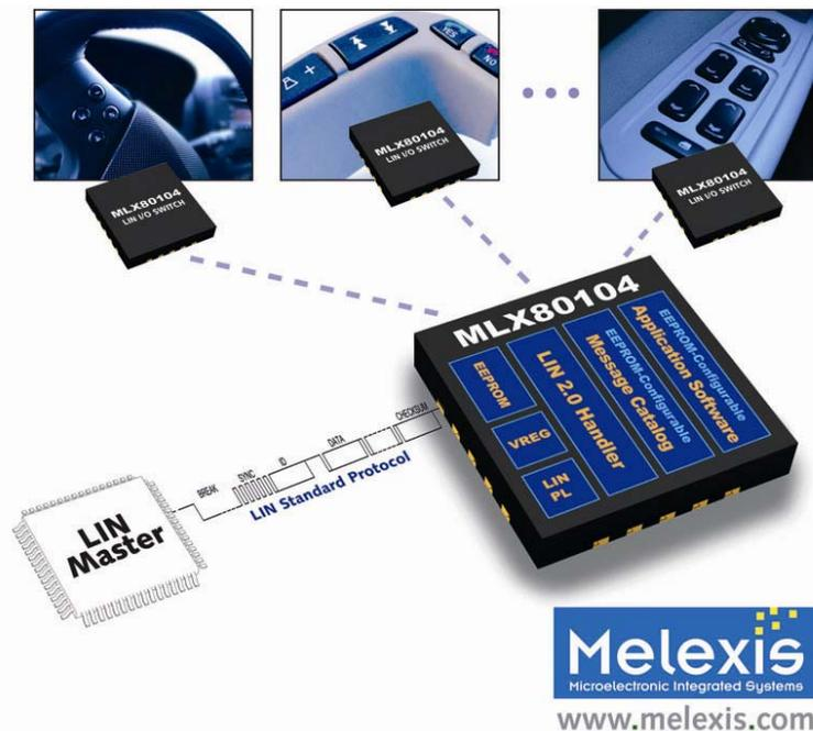
Figure 2 – Definition of a “Plug and Play” LIN Slave
