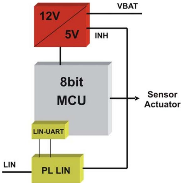
Figure 1 – Block diagram "typical" LIN Slave
