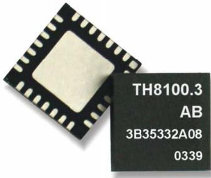
Bus Systems contain specific physical interfaces for automotive busses like LIN, K-Bus or CAN. The new sub-bus system LIN begin its establishment within the current and next car generations. With these physical interfaces the communication on main bus as well as on sub-busses in automotive systems can be realized. Additionally, the 1st products in which these physical interfaces are integrated as embedded blocks in more complex integrated circuits are available.
