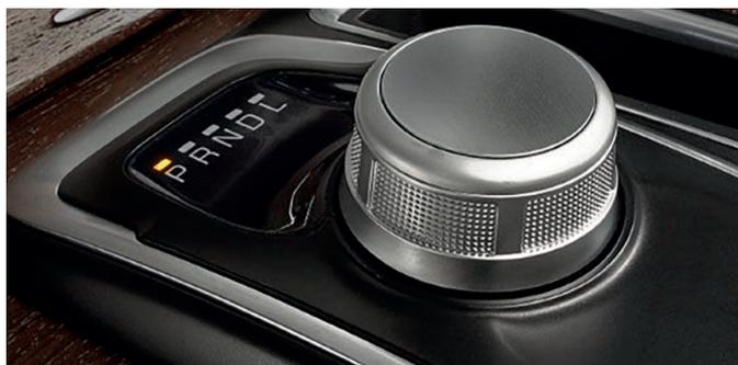
The connection between the shifter and the transmission in an automatic system is using a contactless way of sensing through electric signal (shift by wire).
