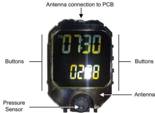
Figure 4-8. eZ430-Chronos Watch Module Front
