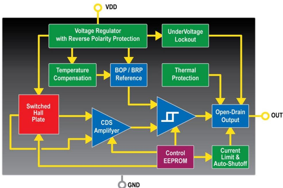
range of  $\pm 0.4\text{mT}$  to  $\pm 80\text{mT}$  and a magnetic switch range of  $\pm 1.5\text{mT}$  to  $\pm 66\text{mT}$  and a programmable hysteresis range between  $1\text{mT}$  and  $36\text{mT}$ . The negative thermal coefficient can be adjusted in the
